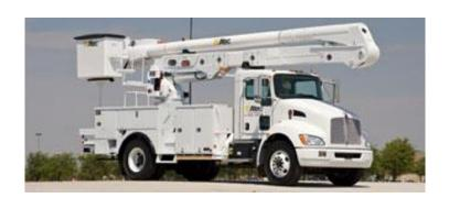
Using a bucket truck can save time and effort, and create a safer environment. However, they must be well maintained. When working with a bucket truck, you must always conduct a daily inspection at the start of each shift to identify any potential problems. Be sure that you follow all inspection requirements and be sure to evaluate the following:
