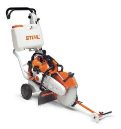
The best way to use a cut-off machine is in a manufacturer-approved cart; hand use of the saw should be avoided. Simple controls allow the operator to adjust the depth and make long straight cuts using water (for dust control). Cutting from a standing position is far more comfortable than crouching (as in hand use)
